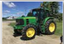
JD 7130 TRACTORS , MFWD, 16 spd, 2 remotes, 540/1000 PTO, 18X38 tires, recent new tires, 6800 hrs Exc cond. Stk# 0862868
