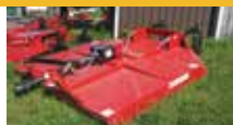
Walco 7' Rotary Mower Unused, 7' Wide, 540 PTO, Slip Clutch, 3 Pt Hitch, 2 Rear Wheels $3,760
