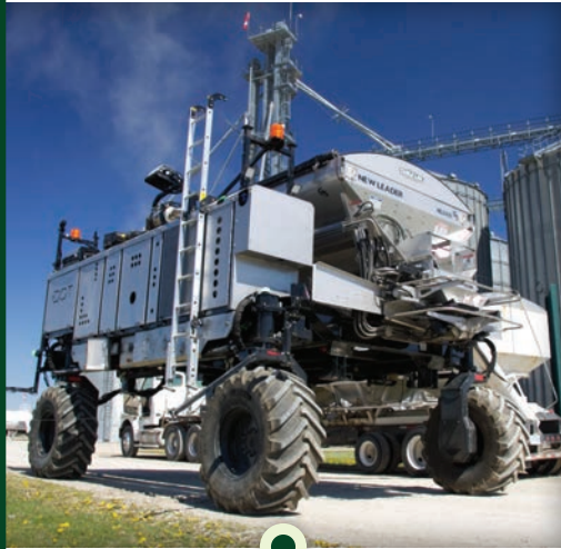
The Raven OMNiPOWER™ completes farm tasks autonomously for a variety of easily interchangeable implements, like a sprayer or spreader.
