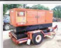
Himoinsa 77KVA generator, Iveco 6cyl. diesel, silent auto start etc
