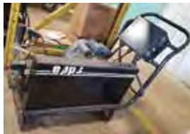
2000 PSI @ 4 GPM. 220V, 5 HP, EPPS Unit, rebuilt, $1000
