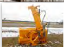
PRONOVOST P-980 TRC snow blower, 8', double auger, truck loading hood, hyd fan turn, 6 blade fan, good cond.
